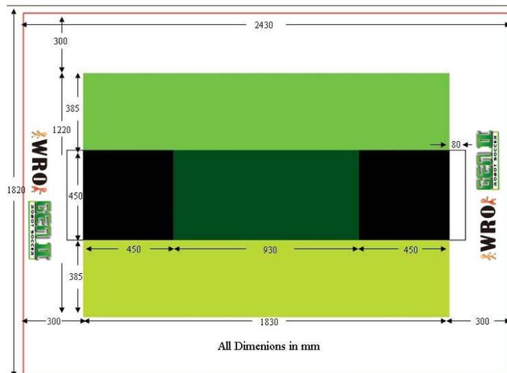
1.1.2. The floor of the playing field is covered with a printed vinyl, roll resistant mat, available from Modern Teaching Aids [http://www.teaching.com.au/lego\\_robotcup.asp](http://www.teaching.com.au/lego_robotcup.asp) or Semia
